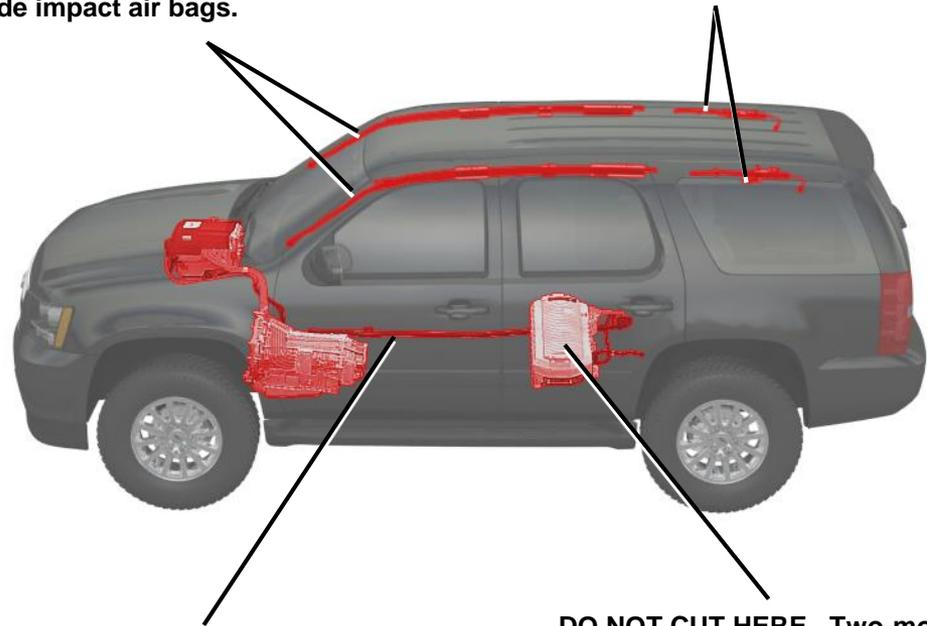
**DO NOT CUT HERE.** Under vehicle area near passenger side frame rail contains high voltage 300 volt electrical cables.
