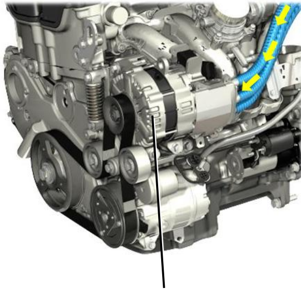
Generator with Starter
